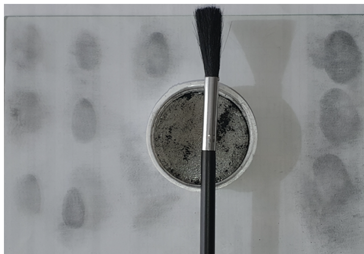
Figure 16 - Dusting fingerprints with fingerprint brush and powder
