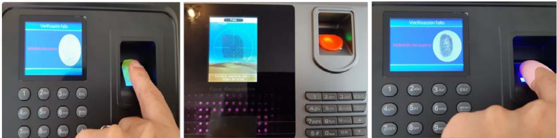
Figure 9 - Experiments with gummy bears, playdoh and silicone fingertips on Hysoon FF395
