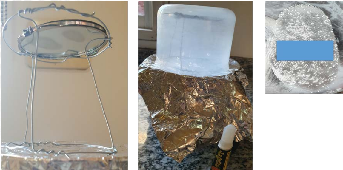
Figure 17 - Ethylcyanoacrylate fuming chamber construction, use and results obtained
